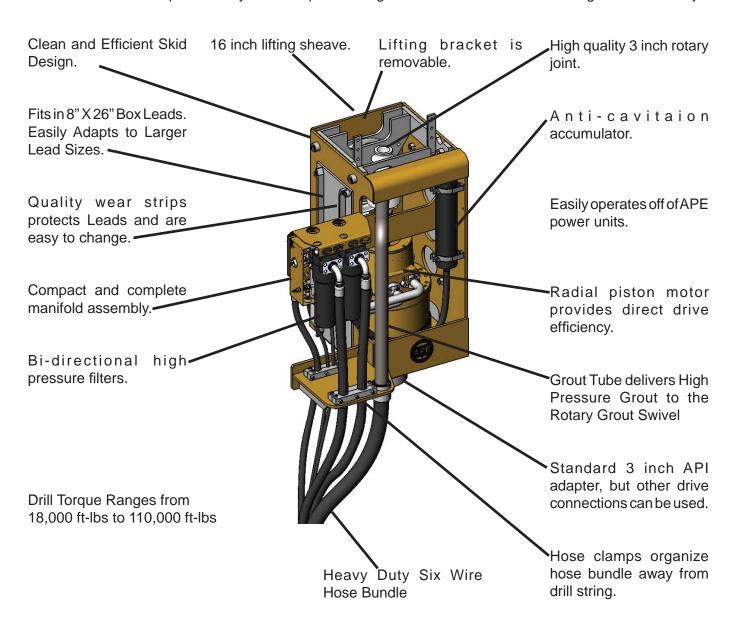
APE provides a full range of high quality hydraulic power units to optimize drill output torque.
